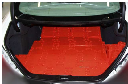
Figure 1. Physical measurement according to DIN 70020
